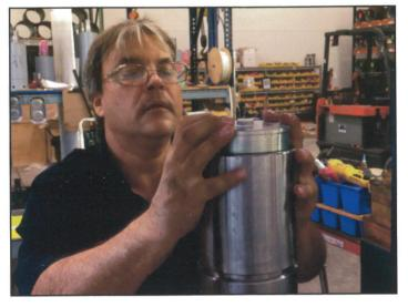
Rulmeca Motorized Pulley diameters of 4.45", 5.45", and 6.49" are most popular in unit handling and food processing applications. However, Rulmeca's complete portfolio includes eleven models, from the tiny 3.15" diameter 0.16 HP unit to the huge 40.16" diameter 330 HP monster. When combined in "multiple drive configuration", conveyor drive power is virtually unlimited.
