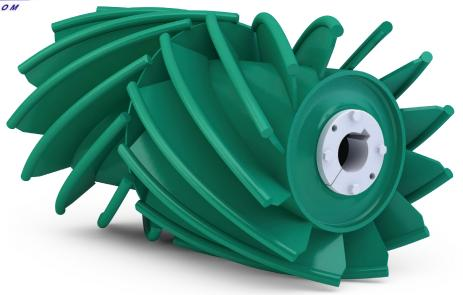
The PPI Herringbone® Wing was designed for those applications where conventional wings suffer from excessive material lodging and wing folding. The extreme wing angles of up to 45®, use the pulleys rotation to eject material out the sides of the pulley rather than recirculating it as a conventional wing often does. These extreme angles and optimized wing height, along with a center reinforcement disc, all combine to make an incredibly strong design that excels where others fail.
